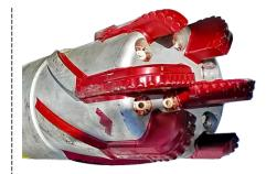
The Weatherford Defyer DPA drillable casing bit has a design—including the nose and blade made of aluminum, and special steel alloy stripe dressed with PDC cutters and secured on top of the aluminum blade—to maximize drilling efficiency, durability, and drillability.
