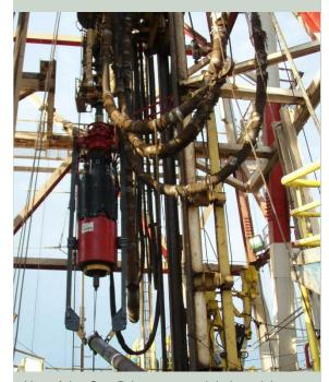
Use of the *OverDrive* system minimizes risk exposure by reducing crew size, including eliminating the need for the stabber. This technology provides faster tubular makeup and breakout without thread damage.
