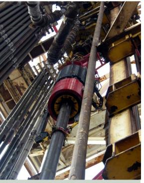
Weatherford's *OverDrive* casing running and drilling system features the *TorkDrive* tool, which greatly enhances safety by combining the functions of power tongs, elevator, fill-up circulation tool, weight compensator, and bails.
