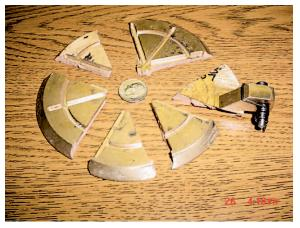
The FLF fluid-loss flapper valve is easily removed at the end of the completion process by mechanically breaking it.
