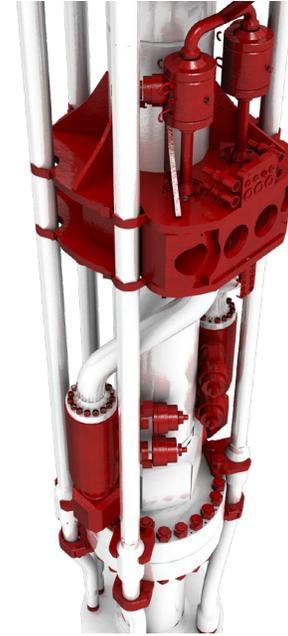
After hands-free installation, the flow spool diverts annular flow to the manifolds on the rig.
