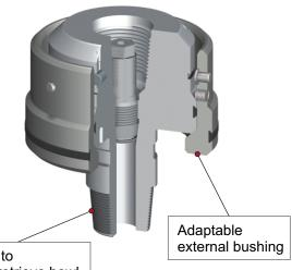
Pin *up* to install/retrieve bowl protectors, *down* to land and seal in head or spool bore
