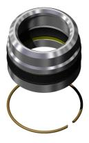
**WFT-PE reducer and seal assemblies** are used as the standard secondary packoff for all WFT casing spools and tubing heads. These parts are pressure-energized and held securely in place with a snap ring.
