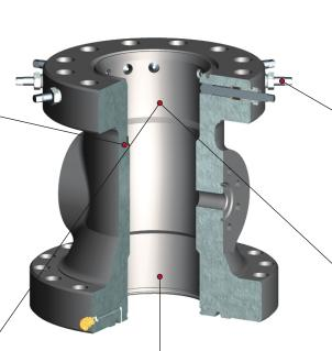
**Connections.** Standard bottom prep for WFT-PE and WFT-4-0 secondary seals. For other applications the prep for WFT-HPPE (high pressure) 15,000-PSI secondary seal is supplied. (Other types available on request.) Externally threaded lockscrews for wear bushing (-BP) and hanger retention (-L) (Example: WFT-22-BP, two lock-screws; WFT-29-L, full set of lock-screws)
