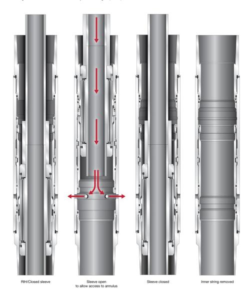
The graphic at left illustrates the mechanical operations of the Eliminator GT Series gastight mechanical port collar model 763.
