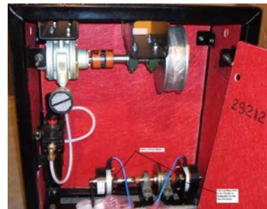
Used with Weatherford surface logging software, the geograph line retriever helps to calculate drilling parameters such as depth and ROP.
