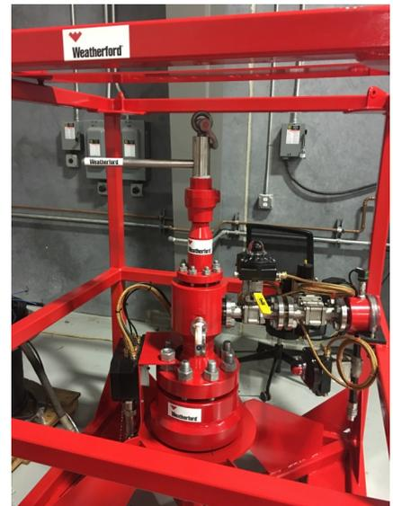
The extraction tree of the MPD fluid-extraction system controls input pressure and closes off the system in the event of over-pressurization.
