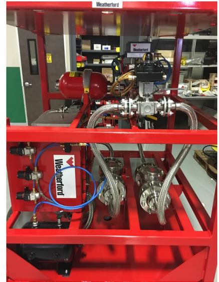
The control module of the MPD fluid-extraction system includes a PLC, which reduces sample pressure to less than 10 psi (0.07 MPa) for conventional gas-detection methods.
