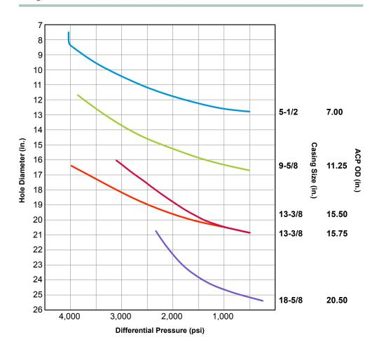
This differential pressure graph illustrates the maximum allowable differential pressure that can be exerted across the element. It is calculated with the packer fully inflated and sealed against the wellbore. Differential pressure is the difference between the annular pressure above the packer and the annular pressure below the packer when it is in the *set* position.
