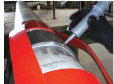
In the image above, a technician injects TubeLok epoxy into the ports of the PoxiLok stop collar.
