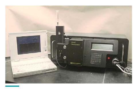
Measurements from the quantitative fluorometer (on the right) can be recorded and converted to weight percent oil and API gravity using a personal computer or laptop.
