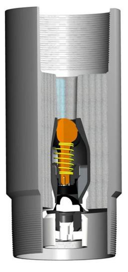
• Cast-aluminum body and rubber-coated seal are PDC-drillable, easing drill out.
