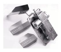
The return flowmeter comes with three paddles to enable use with flowlines of different diameters, and it uses encoder technology to provide accurate measurements in relation to flowline size.
