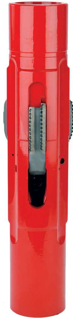
The Weatherford RipTide ball-drop drilling reamer 10625 has retractable and concentric cutter blocks that minimize vibration while drilling and facilitate tool retrieval.
