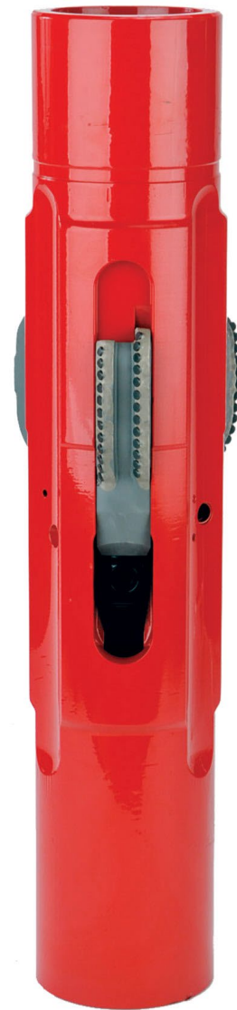
The Weatherford RipTide ball-drop drilling reamer 6000 has retractable and concentric cutter blocks that minimize vibration while drilling and facilitate tool retrieval.
