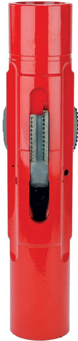
The Weatherford RipTide ball-drop drilling reamer 8500 has retractable and concentric cutter blocks that minimize vibration while drilling and facilitate tool retrieval.
