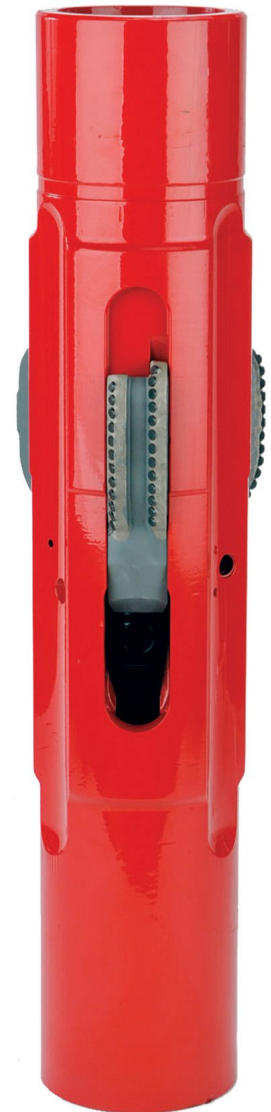
The Weatherford RipTide ball-drop drilling reamer 9500 has retractable and concentric cutter blocks that minimize vibration while drilling and facilitate tool retrieval.
