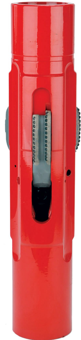
The Weatherford RipTide RFID drilling reamer 10625 has retractable and concentric cutter blocks that minimize vibration while drilling and facilitate tool retrieval.
