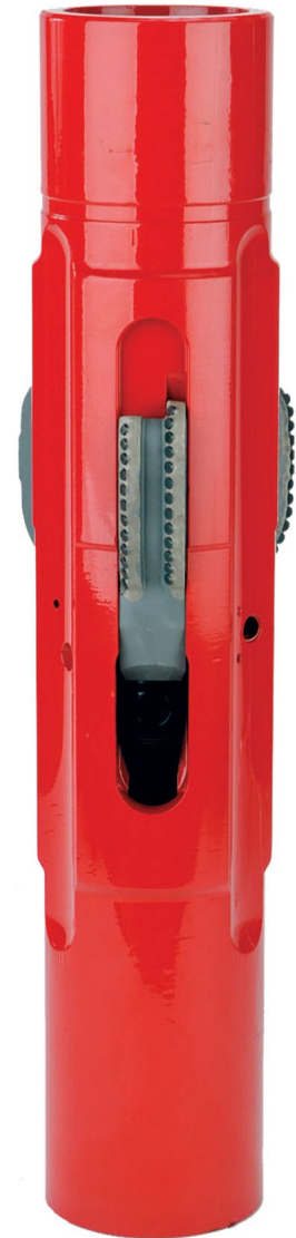
The Weatherford RipTide RFID drilling reamer 12000 has retractable and concentric cutter blocks that minimize vibration while drilling and facilitate tool retrieval.
