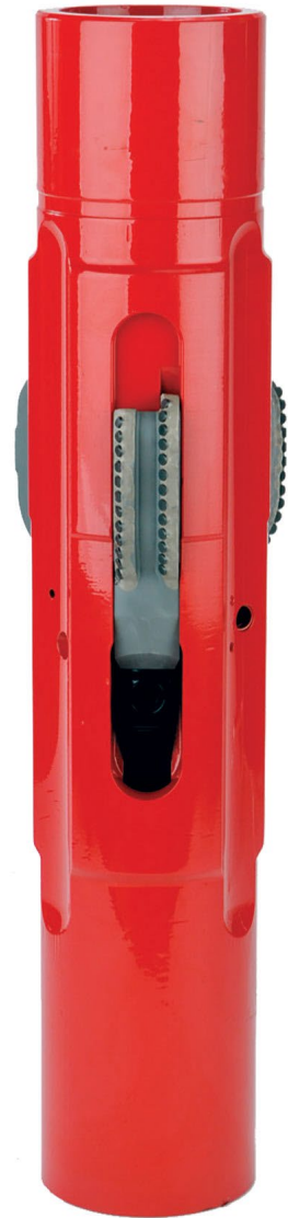
The Weatherford RipTide RFID drilling reamer 8500 has retractable and concentric cutter blocks that minimize vibration while drilling and facilitate tool retrieval.
