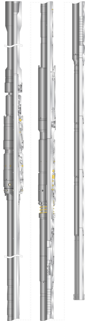
The Weatherford SwageHammer running and setting system (shown above in three segments) enhances reliability by incorporating a surge-resistance tool, a setting cylinder, and a rotating packer actuator.
