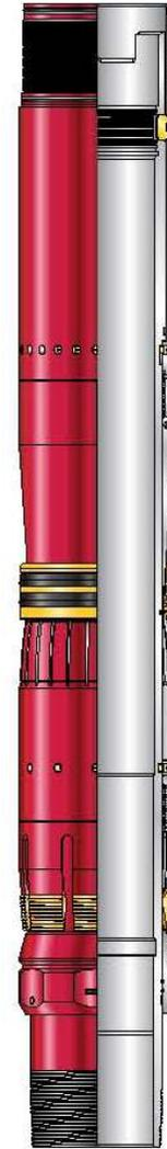
The SwageSet liner-top packer has proprietary swage technology that serves as an annular pressure barrier at the liner top.
