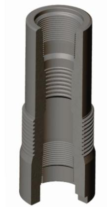
The **WFT-TC-1W slick-joint wraparound packoff** saves time by sealing off the casing annulus while allowing tubing string manipulation/nipping up the tree without blowout preventer (BOP) protection. Tubing weight can be supported on the hanger with a WFT-02 coupling during removal of BOPs. A polished joint is not required.
