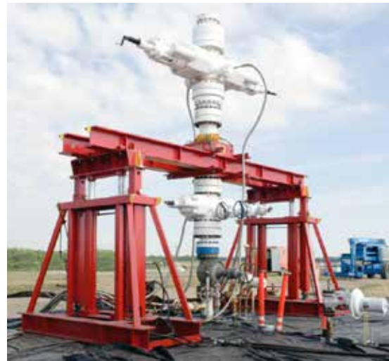
Weatherford engineers configure wellhead support systems based on the specific needs of each location to support the added weight of blowout preventers and other well intervention equipment.
