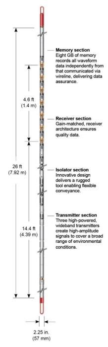
The Compact cross-dipole sonic (CXD) tool enables confident decision making on acoustic reservoir properties using advanced acoustic measurements.
