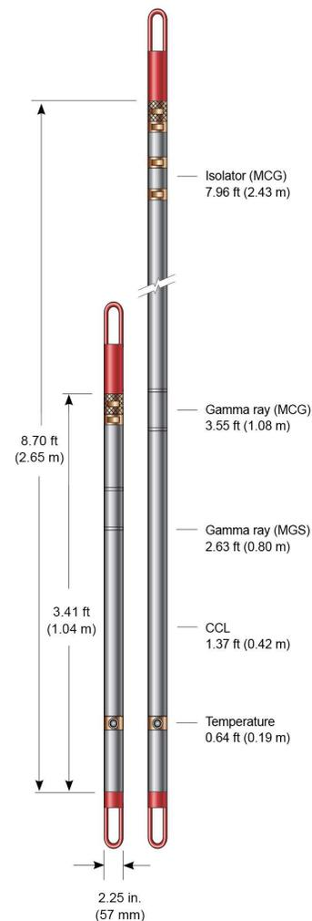
The Weatherford Compact™ gamma ray (MCG) tool provides primary depth correlation for logging tools.
