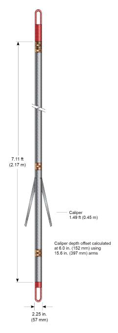
The Compact two-arm caliper (MTC) can be used as a standalone sensor or as a tool-orientation device.
