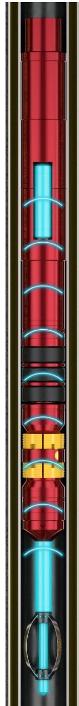
An acoustic sensor (blue) wirelessly transmits P/T data up hole to a data recorder housed in the junk catcher above the plug. The data can be transmitted to surface in real time or can be retrieved from the junk catcher in memory mode.
