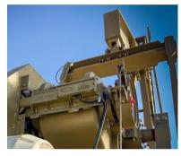
The Atabec safety lock helps maximize safety, minimize downtime, and optimize operational maintenance. Counterweights on beam pumping units can weigh up to 10 tons. The combined weight with momentum and pinch points creates extreme danger to employees.
