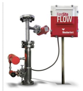
ForeSite Flow VSR is a full-range, non-nuclear multiphase flowmeter that provides complete flow-measurement precision while reducing wellsite complexity, equipment costs, and pad-size requirements when compared with conventional three-phase separators.
