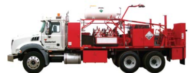
The heavy-duty truck UFW can haul COROD continuous rod to wellsites and provide welding capabilities in the field.
