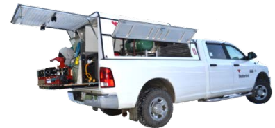
The light-duty truck UFW houses the welding system in the cargo bed of the truck.
