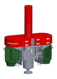
The MG-3750-D electric direct drive is built with a unique centrifugal wet-braking system that provides reliable, controlled backspin protection to enhance operational safety.
