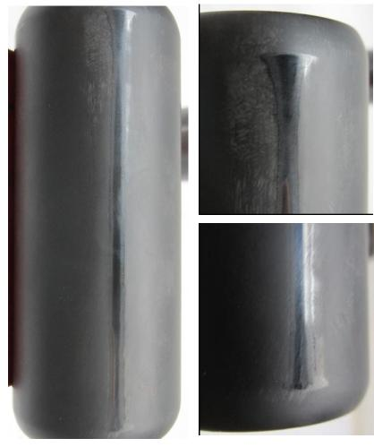
In laboratory wear tests, Racer severe-service couplings show superior wear protection. Following 900,000 strokes with 604b. side pressure, Racer couplings showed only a superficial wear path in sacrificial layer.
