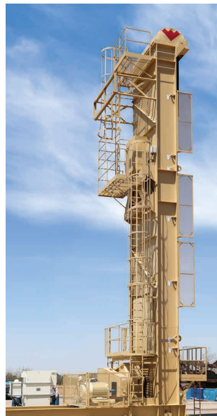
Compared to standard pumping units, the Weatherford Rotaflex long-stroke pumping units improve productivity with a longer stroke, more complete barrel fillage, and less wear on surface and downhole equipment.
