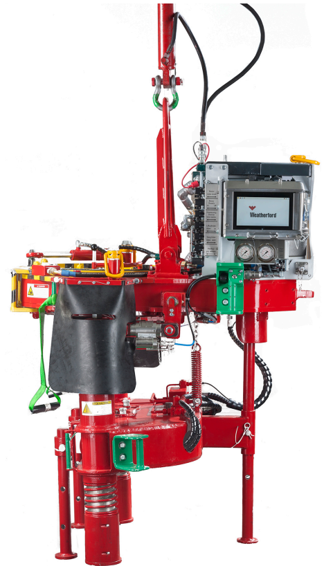
The Weatherford AutoTong system for conventional operations uses a manual power tong in automated makeup applications. After manually positioning the tong to the pipe, the operator pushes a button, and the system automatically identifies components, controls makeup speeds, detects shoulder torques, and evaluates connections.
