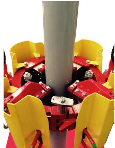
*The four slips on the flush-joint elevator can be dressed to accommodate different pipe sizes.*
