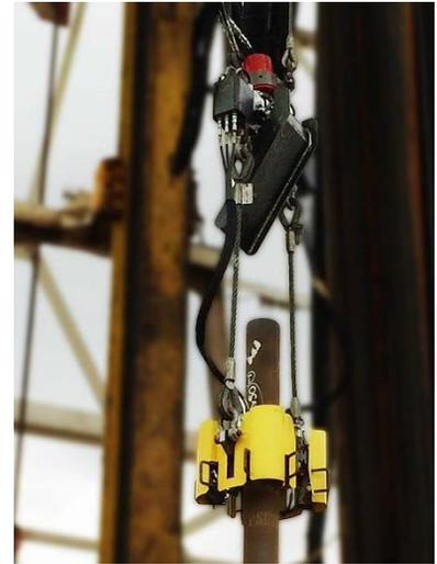
*The flush-joint elevator eliminates the need to thread lift nubbins to lift and make up each joint.*
