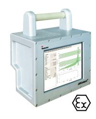
The JAMCompact touch torque/turn system displays real-time data for monitoring makeup and confirming quality connections.
