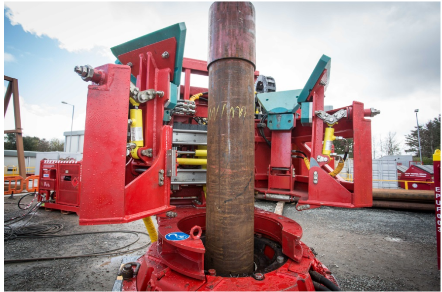
Used in conjunction with the OverDrive system, the Weatherford mechanized stabbing guide enables automated stab-in of tubulars to remove personnel from high-risk zones on the rig floor.
