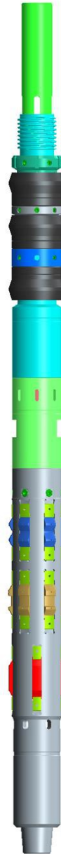
A component of the Weatherford retrievable DwC system, the latch transmits axial and torsional forces from the casing to the BHA or vice versa.
