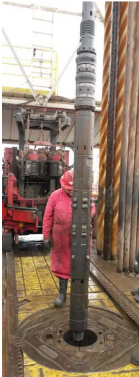
The retrievable DwC latch is always used with the profile collar.
