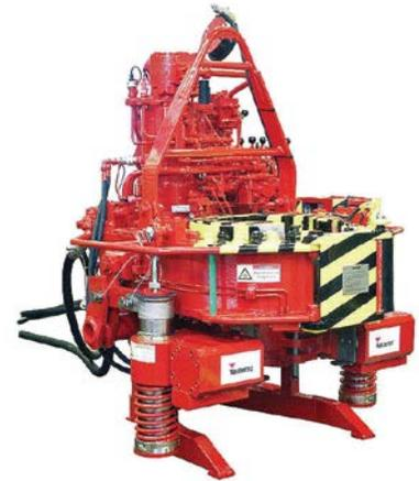
The SpeedTork hydraulic drillpipe tong 8.0-70 enables fully rotational makeups of up to 70,000 ft-lb (94,900 N·m). The tong features a special clamping arrangement to protect the operator and a torsion-bar reaction system to reduce casing deformation.
