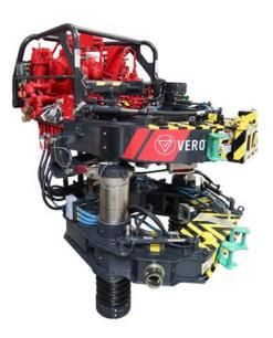
With just a single click from the control room, the Vero mechanized system automates the entire process, from positioning at well center to making up and evaluating the connection
