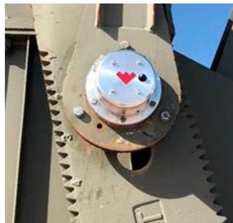
Foresite Sense installs over the wrist-pin cap of surface-pumping units of all major brands.
