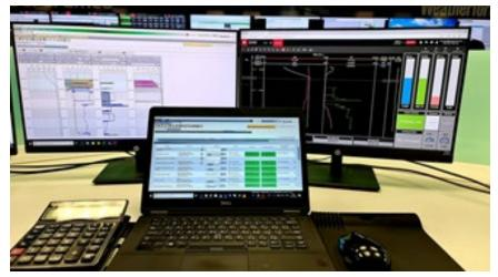
AccuView and Centro systems (displayed left and right) enabled real-time monitoring and close collaboration between the rig and offsite support team.
