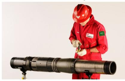
The SwageSet system is prepared for installation.
