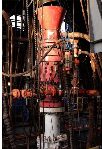
The Weatherford SeaShield Model 7875 DS RCD enabled PMCD through a hazard zone to mitigate drilling-fluid losses and enhance drilling efficiency.
