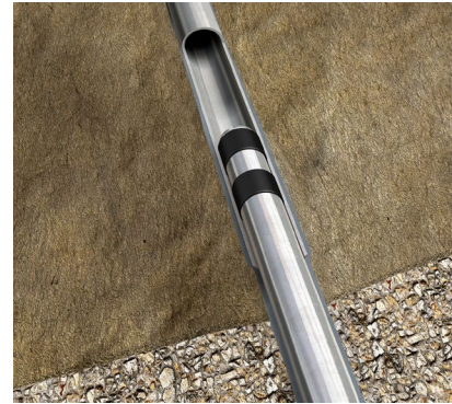
Weatherford coordinated services from multiple product lines to isolate older perforations from the main wellbore.
