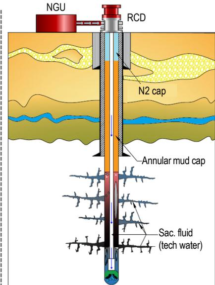
Weatherford introduced a nitrogen storage system with a nitrogen-generating unit on the location. The system connected to the well via the kill line to deliver instant nitrogen for nitrified PMCD operations.
