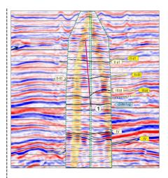
Walkaway VSP data (center) is superimposed on surface seismic data to show improved detail and to aid in depth correlation
